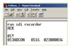
Figure 9 –TBS03 Transfer mode, sensor response on ID command 0!!
