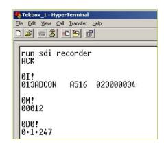
Figure 11 –TBS03 Transfer mode, sensor response on Send Data command 0D! Other SDI commands will work similarly.
